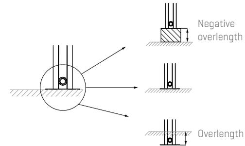
Positive overlength is possible up to the maximum passage height [9' 6 11/64"] plus 1' 7 11/16" [11' 1 55/64"].
