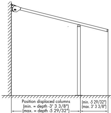
A shifted column in Lapure must be entered by entering the required distance from the wall connection.
