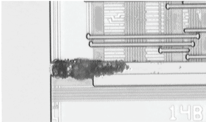
Figure 5.11 A Trace in Integrated Circuit Damaged by Electrical Overstress (EOS)
