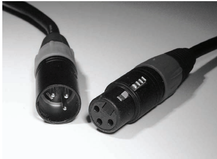
The common 3-pin type, male plug (output) is on the left; the female receptacle (input) is on the right.
