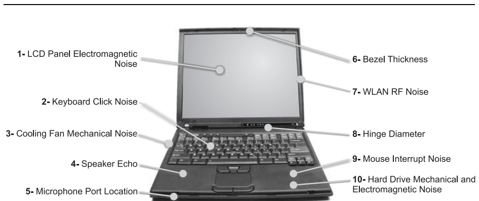
Figure 5.6 Noise Sources Affecting Microphone Placement in a Mobile PC
