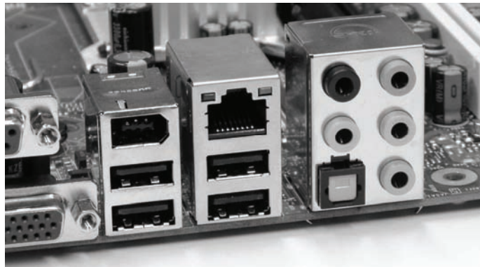
Figure 2.16 Color coded jacks on a typical Intel HD Audio motherboard.
