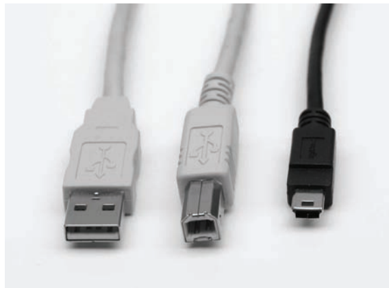
In order from left to right: Type A, Type B, and Mini USB.
