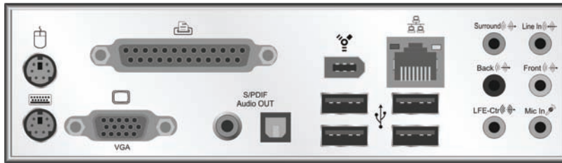
Productivity PC with six 3.5-millimeter jacks and separate S/PDIF connectors
