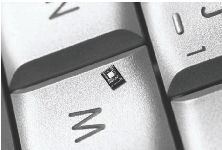
A single chip contains the transducer, analog preamplifier, and an analog-to-digital converter. (Courtesy of Akustica®)
