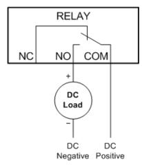
By default, the relay output turns on each time the XL Display goes into Down mode. The relay output turns off once a Down reason is scanned. The operation of the relay can be changed if this is not the operation that you desire. Give us a call if you need to change the operation of the relay output.
