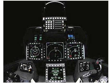
Cockpit of the F-22, showing instruments, head-up display and throttle top (lower left)
