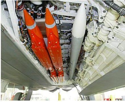
One AIM-120 AMRAAM (right) and four GBU-39 SDB (left) fitted in the main weapons bay of an F-22
