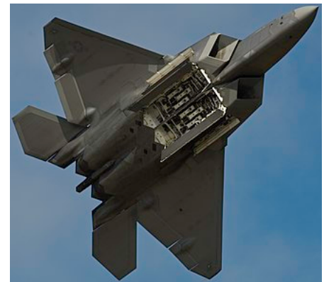
F-22's underside with main bay doors open
