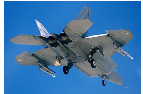
F-22 with external weapons pylons
