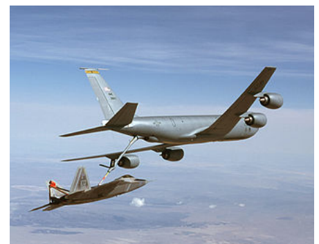
An F-22 refuels from a KC-135 during testing; the attachment on the back top is for a spin recovery chute
