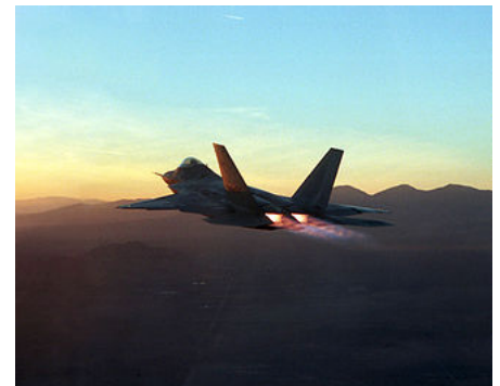
F-22 flying with its Pratt & Whitney F119-PW-100 engines on full afterburner during testing
