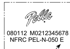
The letter E on the glass identification label indicates SunDefense Dual Low-E glass.
