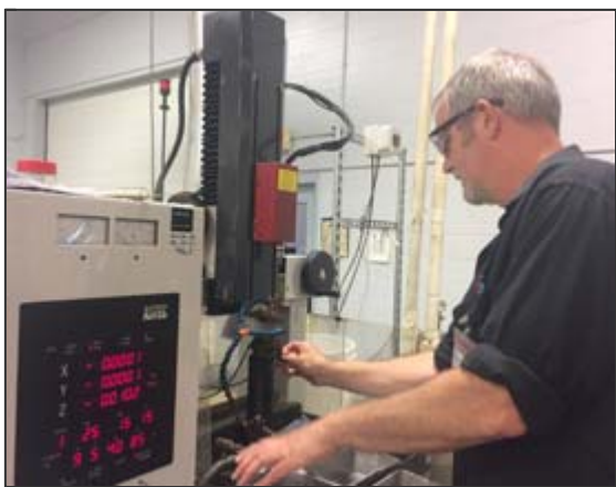
An apprentice in a HITEC apprenticeship program at Vermont Precision Tools operates an electrical discharge machining (EDM) drill to create very small precision holes on the end of a long thin part. EDM is a very precise material removal process that works on the principle of using an electric arc
