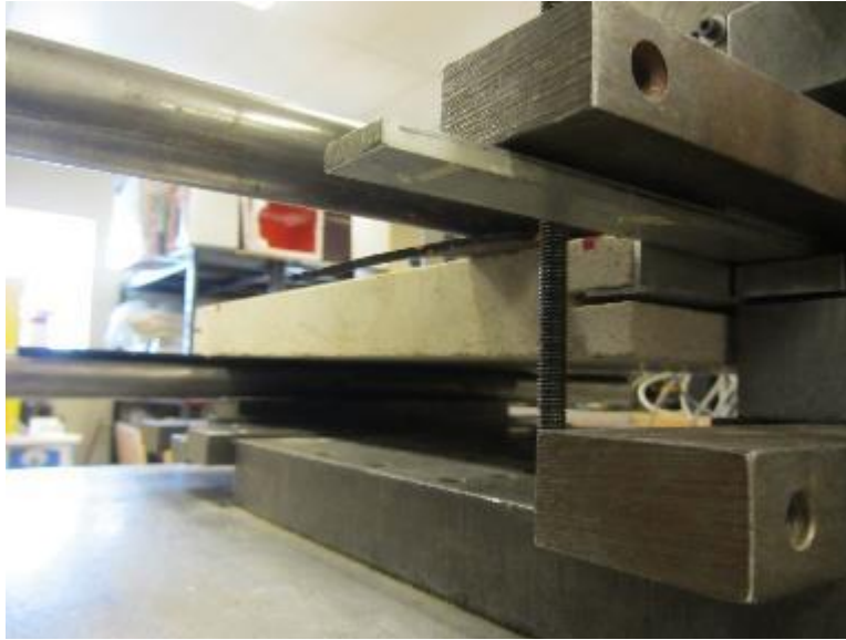
Photo No. 5 ASTM C1354 - Kerf Lip Loading Detail
