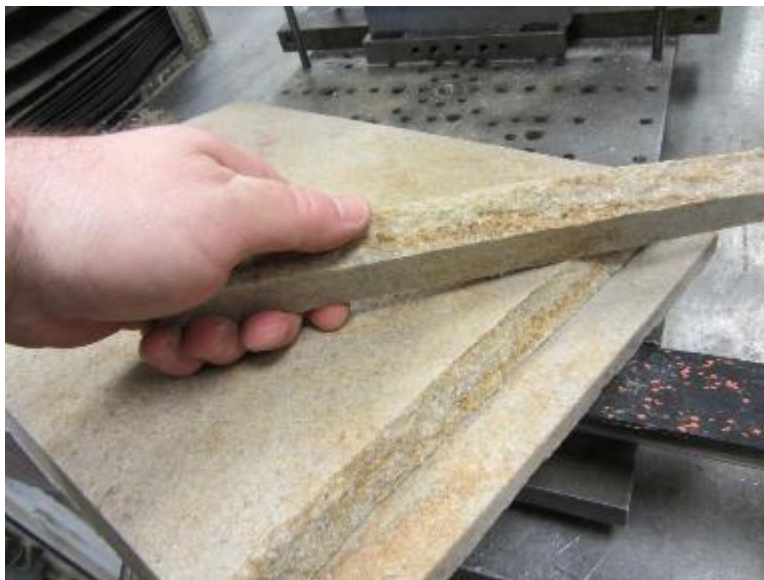
Photo No. 6 ASTM C1354 - Representative Kerf Mockup Failure Mode - Stone Fracture (Kerf Lip)
