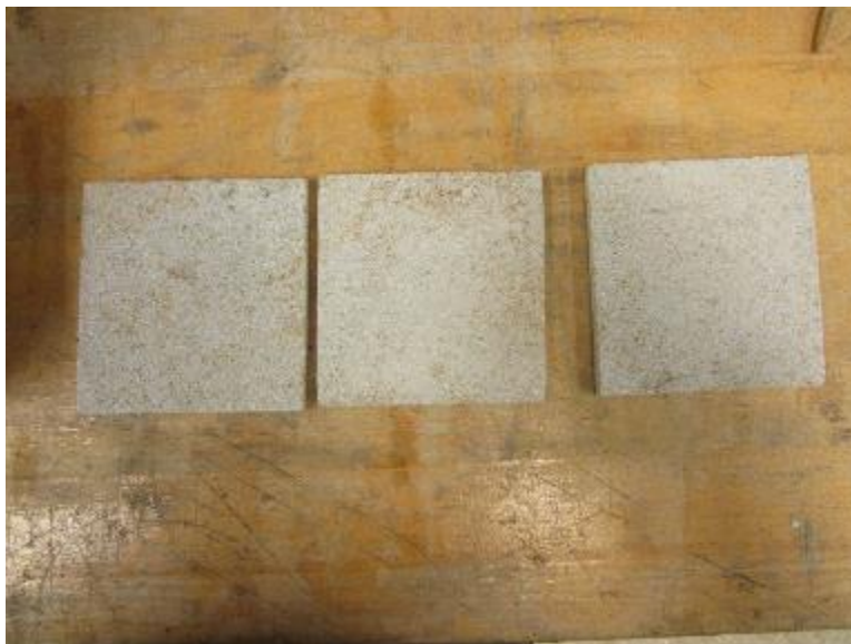
Photo No. 8 ASTM C1353 Abrasion Resistance Test Specimen Post-Test Condition
