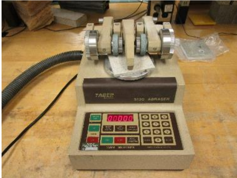
Photo No. 7 ASTM C1353 Abrasion Resistance Test Apparatus
