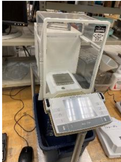
Photo No. 2 ASTM C97 Absorption/Density Evaluation Test Apparatus (Immersed/Suspended Mass Determination)
