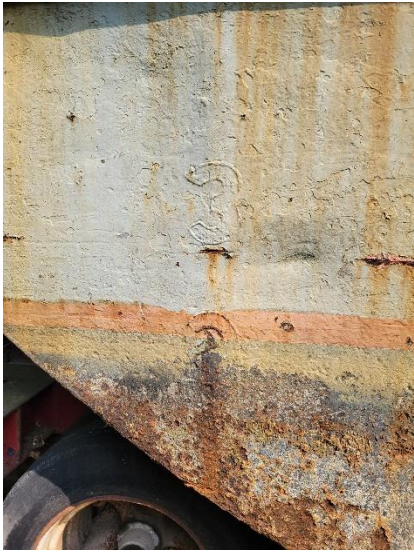
Recent photo showing the current colors as well as the two and three-foot markers that were welded onto the hull. The hull is marked like this in four places.
