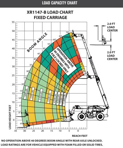
LOAD RATING INCLUDES WEIGHT OF ANY RIGGING. 5,500 LBS AT 24 IN MIN CAPACITY FORK (11,000 LBS PAIR).
