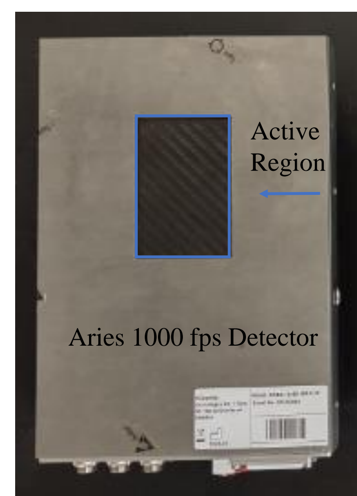
Figure 1. (Left) Carotid waveform used for pulsatile anatomically-realistic flow. (Right) 1000 fps CdTe 100 \mu\text{m} pixel pitch single photon-counting detector (Aries, from Varex).
