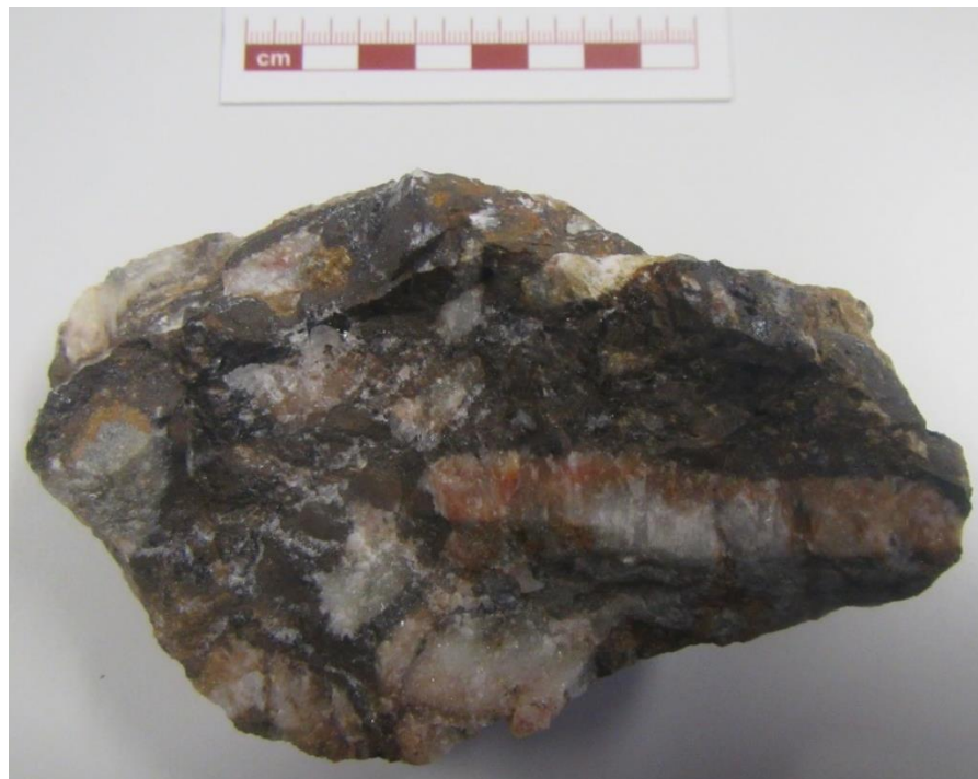
Iron oxide matrix fault breccia, Lacey's Tank Prospect (MGA 94 zone 55 532614mE 6439259mN)
