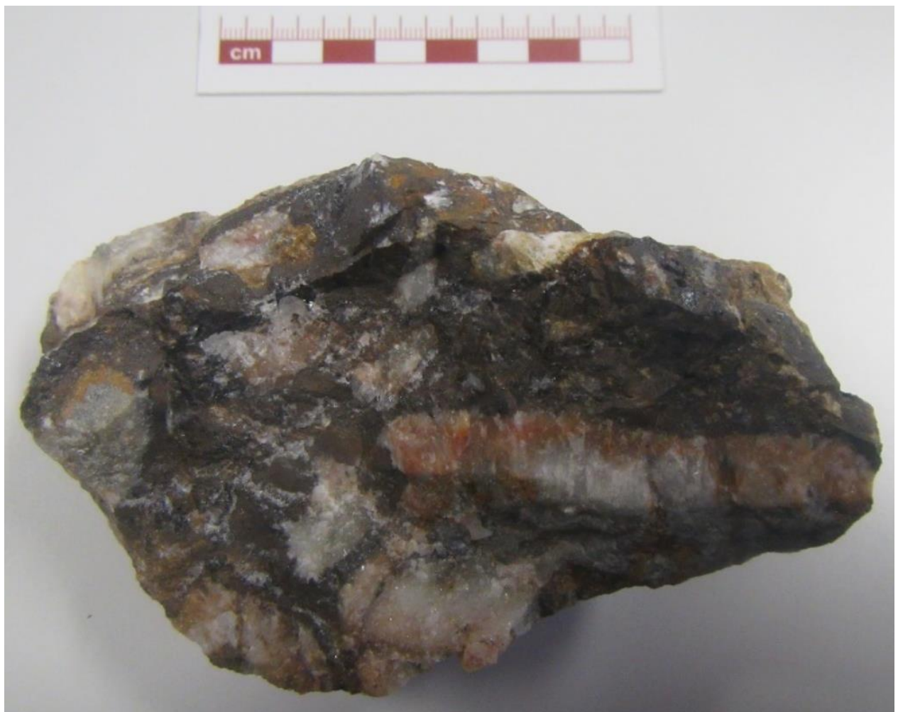
Sample IC220826-11; Iron oxide matrix fault breccia, Lacey's Tank Prospect (MGA 94 zone 55 532614mE 6439259mN), 0.38ppm Au, 0.18% Cu
