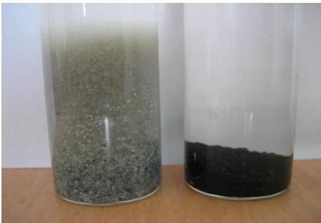
Dissolved FCMP 0-8-0 in citric acid with a Silicate "FLOC" (left) and insoluble in water (right)
