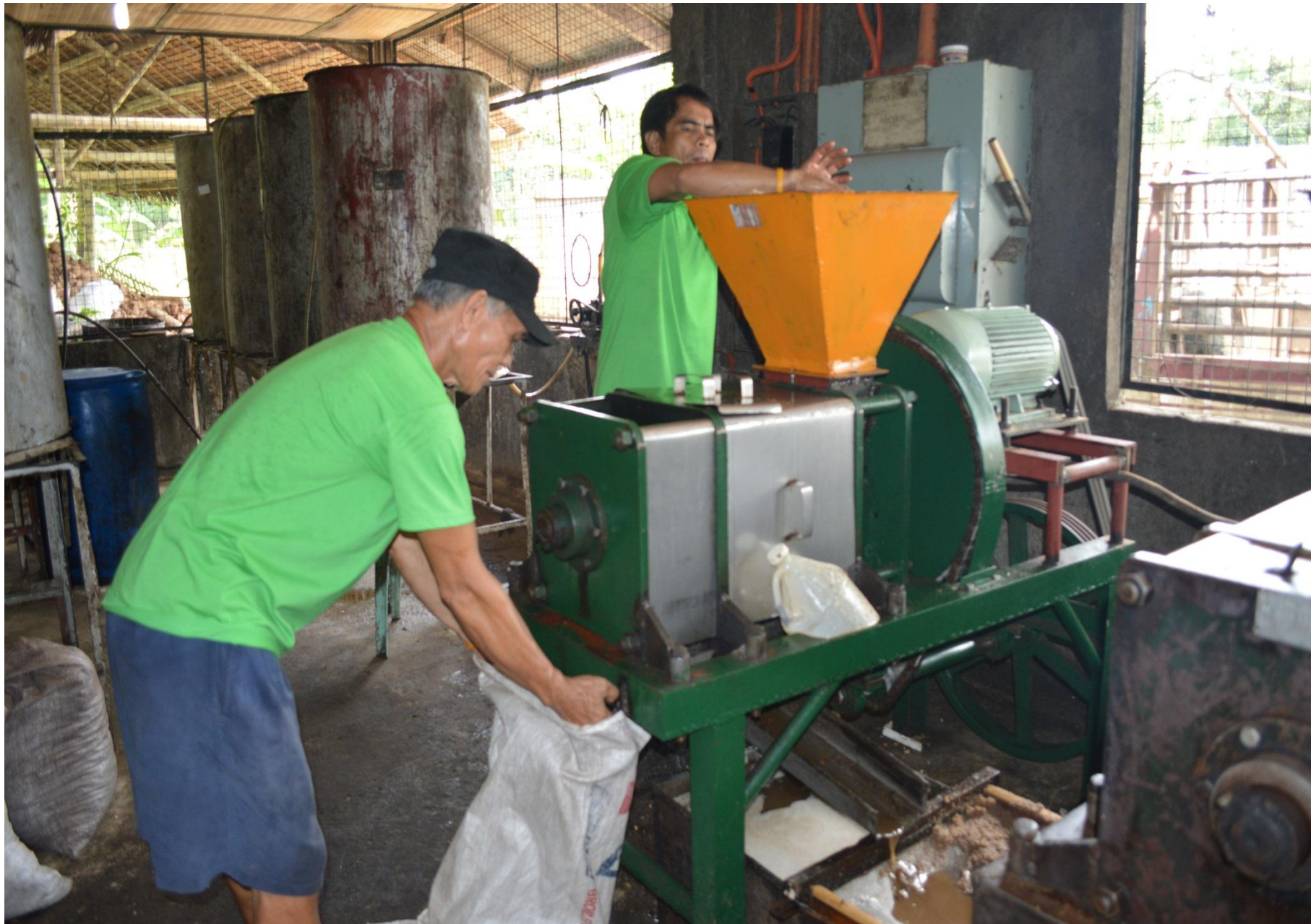
CASCOFAMCO Workers Operating the newly installed Coconut Oil Expeller
