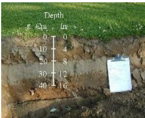
Figure 2-4. The sand layer between 20 and 30 cm depth effectively blocks upward capillary flow.
