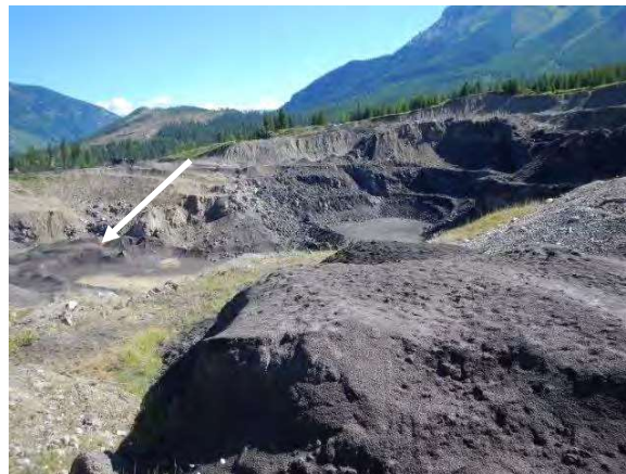
Figure 7. The inactive quarry showing the patches of grass with no thistle. There is a “fines pile” indicated by arrow which may be removed and processed. See Appendix 1 for location.
