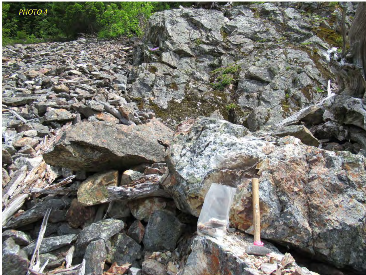
Photo 3 A sample was collected from mineralized quartz talus boulder carrying finely disseminated arsenopyrite with GPS waypoint sample RCZ-05
