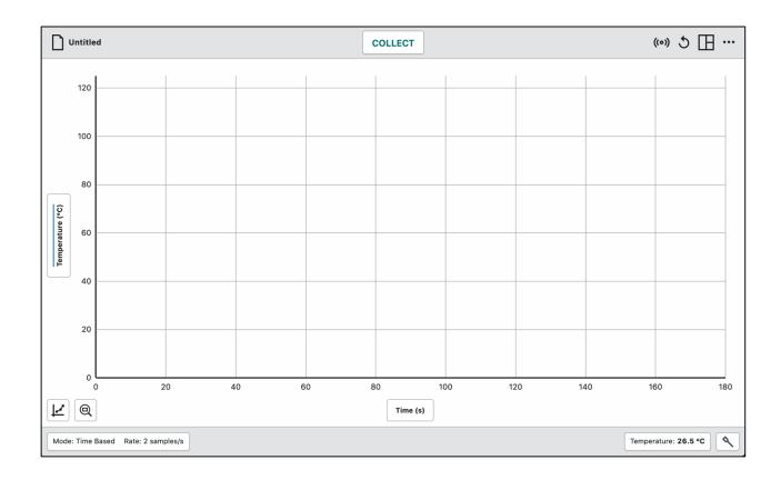
Each time you hit the **Collect** button, a new data set will run. Click on the label on the y-axis to select which data sets are displayed. Check and uncheck boxes to display various data
