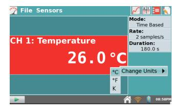
It is easy to change the units, by clicking on the red "meter". A pull down menu will appear to allow you to specify units. Some sensors will also have an option to zero the sensor.
