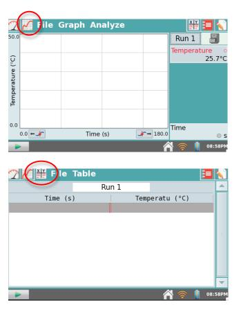
The default setting will be a **Time Based** experiment, which means that the data will be collected over time. If you wish to change the time that the experiment will last, sampling rate or to change to a different mode, click on the table showing **Mode, Rate, Length** (be sure you are at the main "meter" screen). A new
