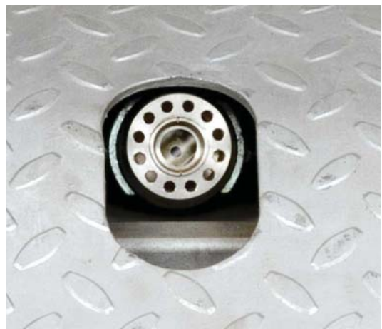
Rugged camera modules have high-intensity bright white LEDs built in.
