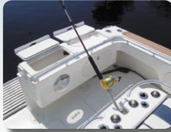
42 gal. Live well/Sink/1500 lb. Pressure Washer
