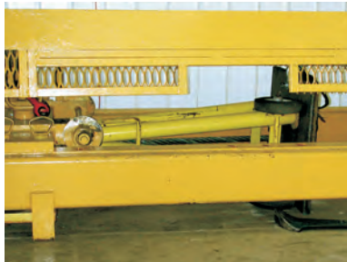
Positioning the railroad car stand in LiftPRO's 300,000 lb. Test Bed - preparing to test
