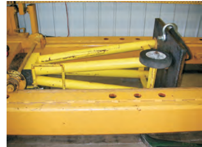
Testing and Certifying each railroad car stand to 147,000 lbs. per stand
