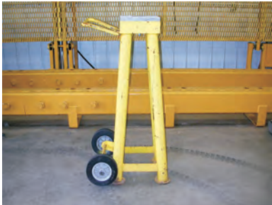
Railroad car stand submitted to LiftPRO for ASTME E4 Testing and Certification
