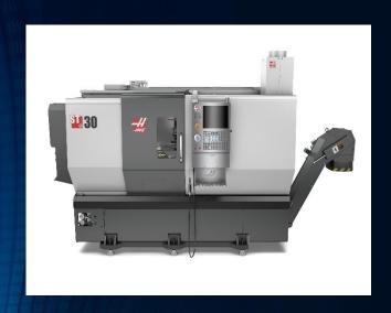
The ability to turn and mill complex parts and perform multiple operations on a single machine increases throughput, reduces handling, and improves part accuracy. The Haas ST-30 Series Y-axis turning centers provide 4" of Y-axis travel (±2" from the centerline) for off-center milling, drilling, and tapping, and come standard with high-torque live tooling and a servo-driven C axis for versatile 4-axis capability. They are available in standard and Super
