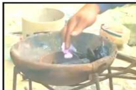
PREPARATION FOR MELTING The cloth containing the amalgam is placed in a crucible.
