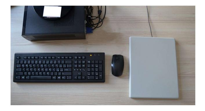
The shielded workstation provides staff with a quick and efficient solution to program and verify RFID tags. The library staff can also activate / deactivate the anti-theft of documents without the direct use of the management system in use.
