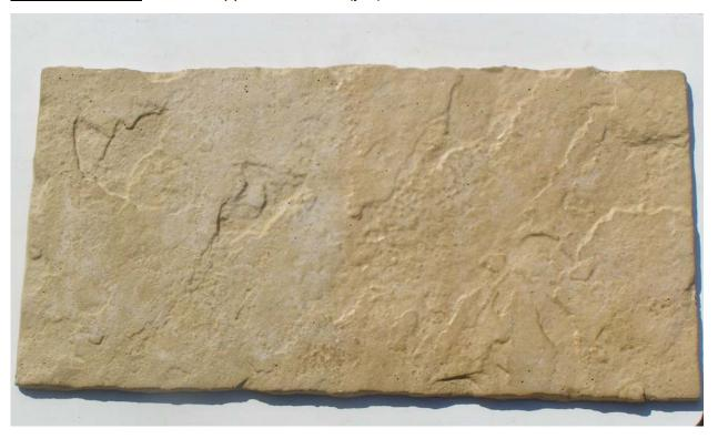
This thin uniform casting demonstrates the extremely lightweight, low profile in a Sand Stone finish, which can be cast in differing colors and hues to help accentuate the finer rock face details. The overall weight of this piece 3.3 pounds at 23" X 11.5" (2 Sq.Ft installed) which averages 1.65 pounds per Sq.Ft.
