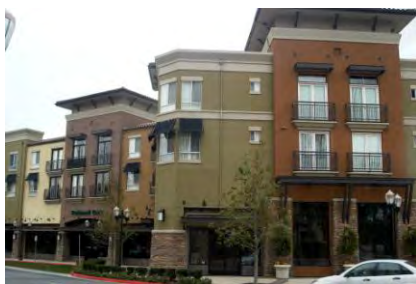
The use of different colors, materials, and other façade elements help break building mass
