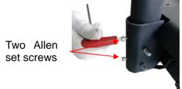
Extend the handle bar tube to full upright position, and slide it into connecting with the front fork.
