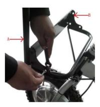
4. Install the rear frame onto the scooter with the two bolts, and tighten them with the nuts provided.
