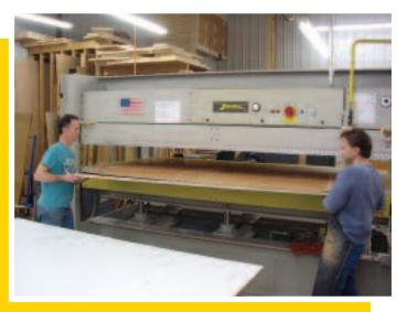
The addition of the Joos HP-150 Okotherm water-heated press has given Wall/Goldfinger added capabilities for pressing large panels, while reducing its production time by half.
