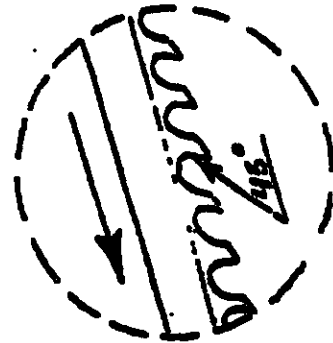
Install all nozzles so the MerLube hits the face of the tooth (gullet).
