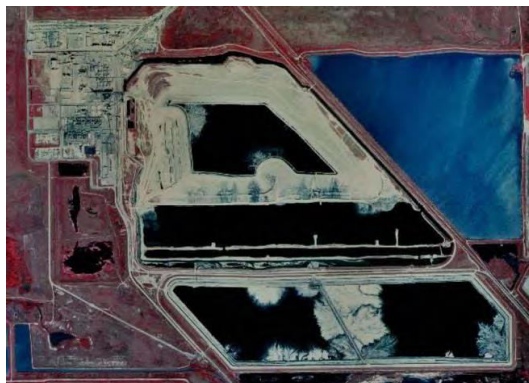
Figure A. Aerial Photo of a chemical plant and its associated gypsum stacks and cooling water ponds.
