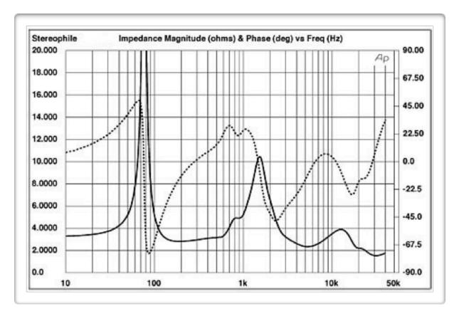
The black line is the varying impedance of the loudspeaker at different frequencies and the dotted line is the phase curve.
