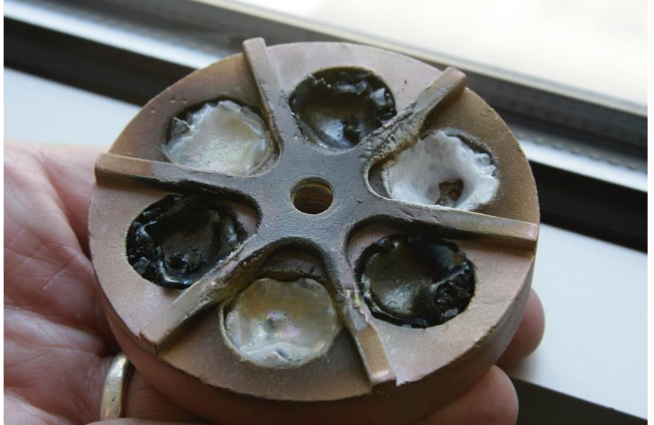
This disk of rare-earth anti-reflection minerals supplies the anti-reflection coatings applied via electronic vapor deposition.
