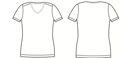
Deep V Collar Short Sleeves Front Shoulder Fold Cuff Lock Stitch - Girl's Cut
