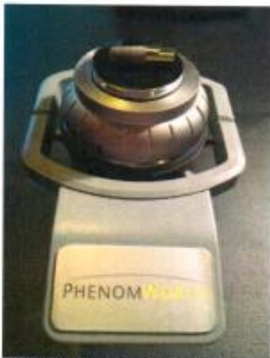
Fixed implant on the sample holder (example)
