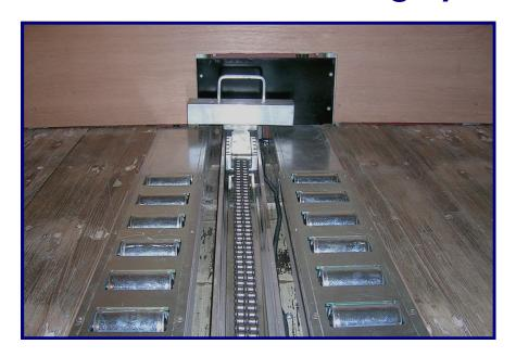
The Rollerbed Systems T-Bar Off-Loader is a vehicle mounted off-loading system aimed at those users carrying palletized loads such as empty food or beverage cans, glass bottles or finished products. The system is mounted flush within the floor of the trailer to maintain continuity with standard loading docks. The single chain drive unit is mounted centrally at the front bulkhead to provide a direct
