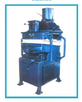
"UMAS" Destoners are fully enclosed for dust free operation. Easy to operate controls are provided for feed, speed, pitch, elevation and air.
