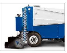
**Integrated Auger Washout System** Simplifies the vertical and horizontal auger washout task, from a single point on the conditioner.
