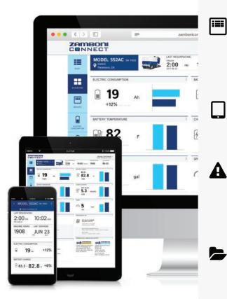
WiFi Requirements: WiFi router with a minimum signal strength of -70 dBm and is compliant with IEEE 802.11 b/g/n. A dedicated router for Zamboni Connect" system is recommended. Best location for router installation is in machine storage room, or line of sight to machine storage room or ice pad.
