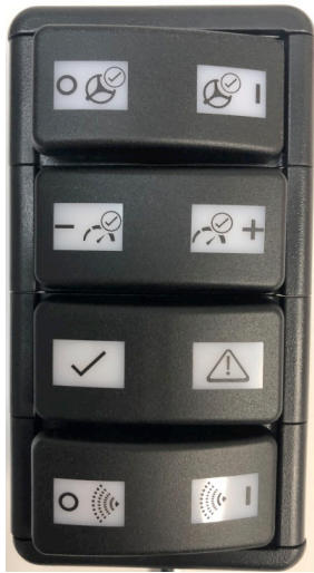
Figure 2: FastICE Switch Bank 1 switch and LED identification
