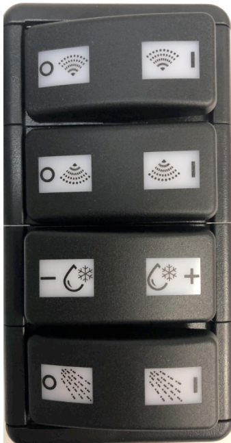
Figure 3: FastICE Switch Bank 2 switch and LED identification
