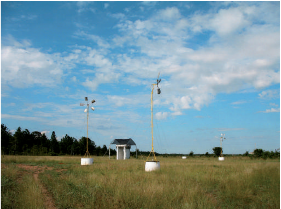
Extraction of GAVIOTAS natural tropical water by windmills with double effect above the springs
