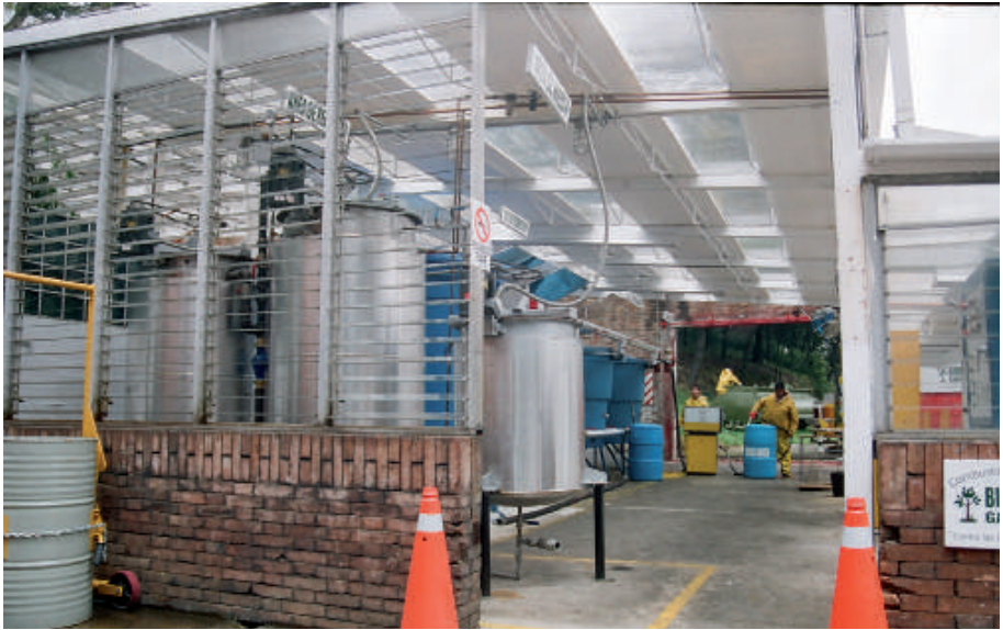
GAVIOTAS type biodiesel plant using crude Africa palm oil located in Bogota. Currently biodiesel is extracted from the tropical caribbean pine oleoresin
