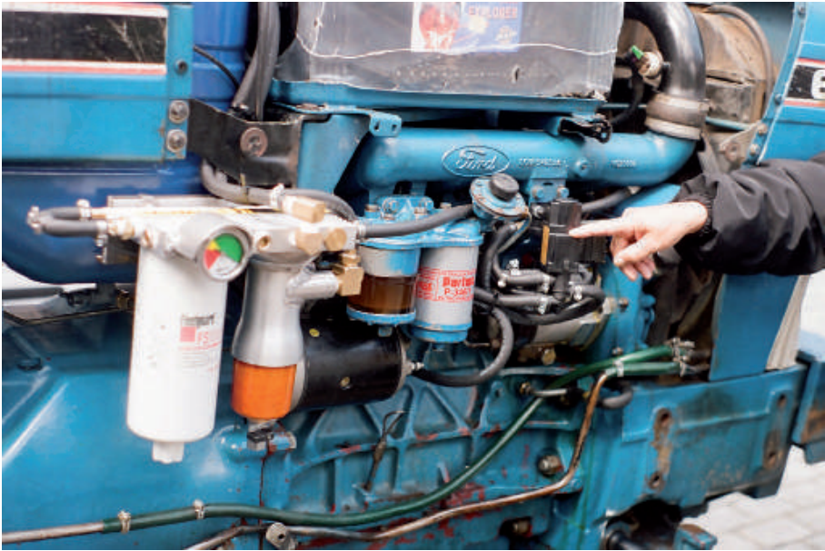
Appearance of a tractor operating with crude African palm oil to which was added an outdoor oil heating kit
