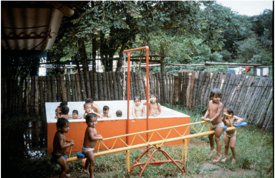
GAVIOTAS see-saw pump for water extraction
