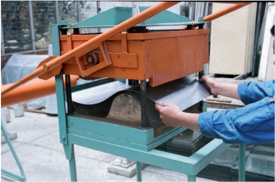
Manual machine for bending sheets used in GAVIOTAS tropical double effect windmills
