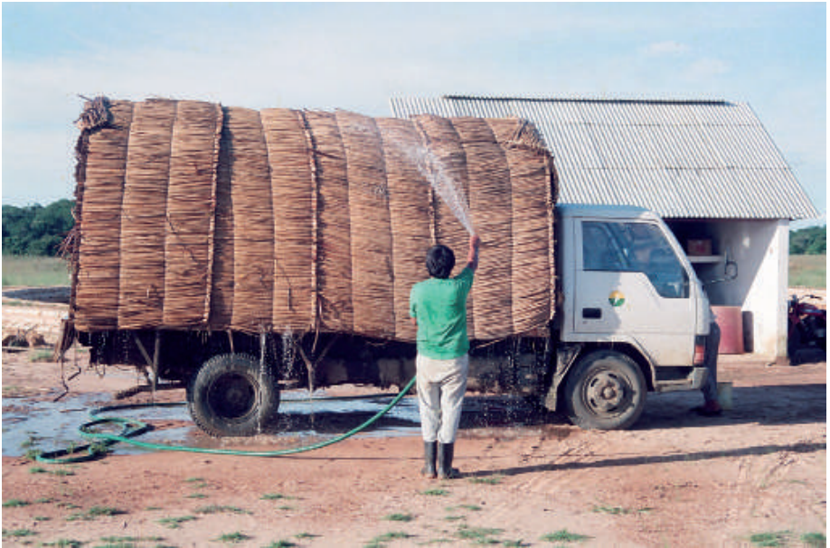
Appropriate technology for cooling the truck transporting the tropical caribbean pine seedlings
