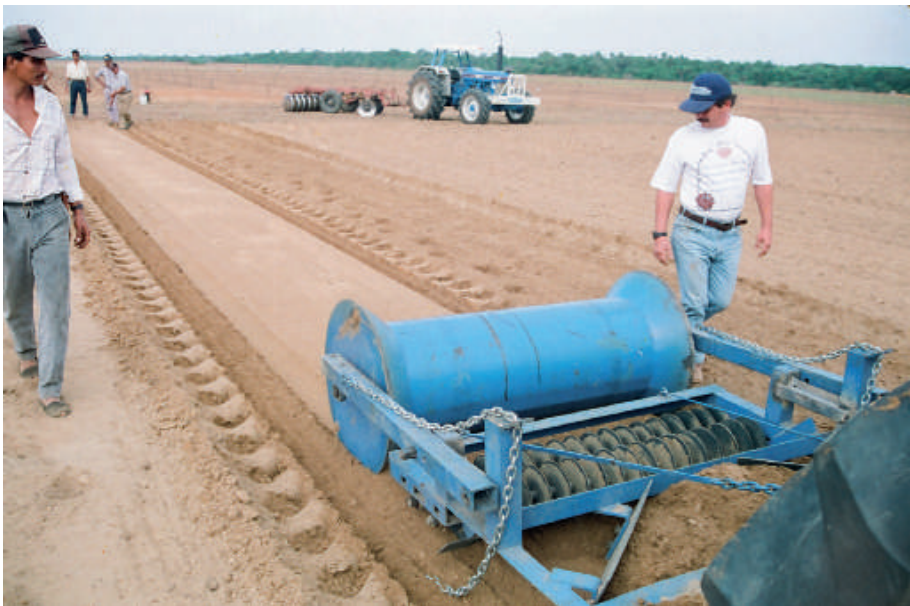
Machine for constructing terraces in the tropical caribbean pine nursery at GAVIOTAS
