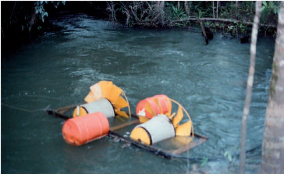
GAVIOTAS hydrostatic pump to draw water
