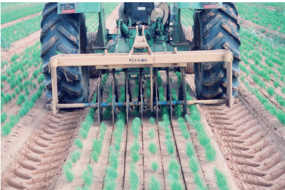
Lateral pruning of the roots of tropical caribbean pine seedlings in the nursery, GAVIOTAS
