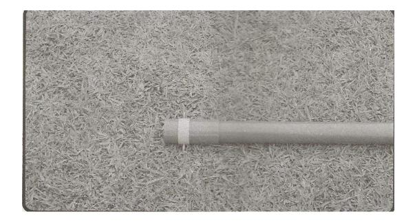
The galvanized pipe is joined with screwing fittings
