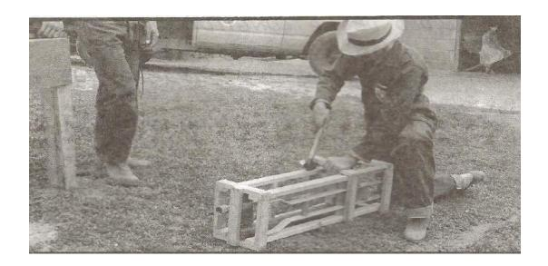
Get used to the parts of the pump, but do not ensemble the head before you have drilled the well, the support for the pump and having all the materials for the pipe, the sleeve and the feeding hose.
