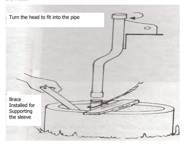
After connecting low down the head and fix it on the support with some screws or nails up to 5" long.
