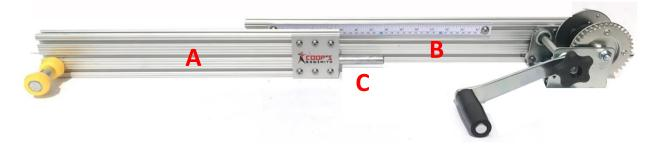
Slide parts A and B together. Slide joiner plate aligning index mark with the center of the 2 main pieces.
