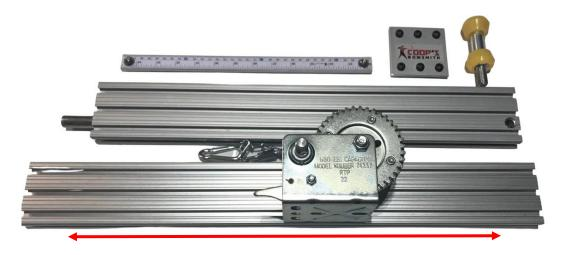
Losen the 3 screw and slide the winch to the side and lock in place.
