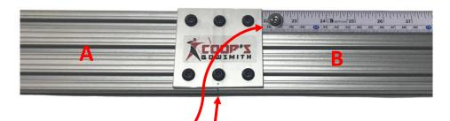
Align the index mark on the center of parts A and B and tighten in place. slide the draw scale so it touches the side of the joiner plate.
