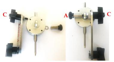
Install the dial gauge in this manner.Inside the knob is a button head cap screw (C). Hold the screw while you tighten the thumb screw (A).Do not remove the inner nut (its Loctite), bushing or washers.
