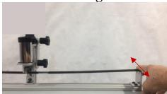
With the weight on the pan simply roll the shaft. You will feel it roll into a valley. It's easier to apply a little more weight to the pan by pushing the weight down with your left hand and rolling the shaft with your right. The shaft will flex towards the weak side down. Rotate the shaft 180 degrees and mark the shaft with paint, this is where you want the top of the shaft to be.
