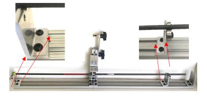
NOTE: alignment holes for 28 inch or 26 inch set up.
