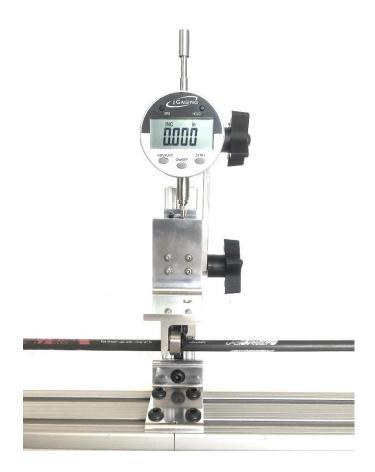
Zero the gauge - add the weight and read deflection. Note: a couple lite taps may help to stabilize the gauge.
