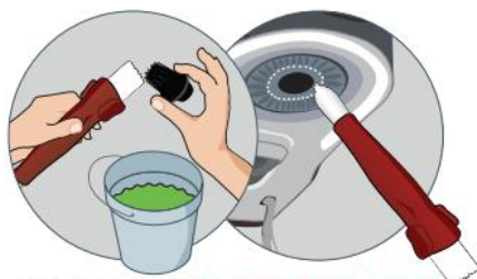
clean, then sanitize the nozzle & injector ring you must soak the nozzle tip with food grade sanitizer. Then allow to air dry for 2 minutes
