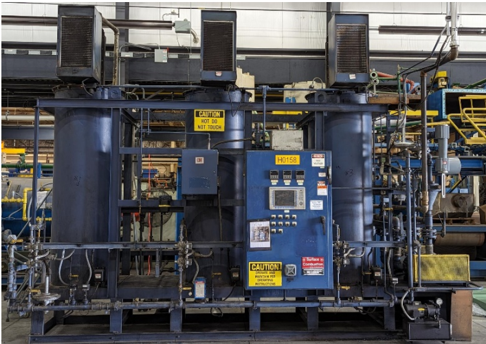
E-155 6,000 CFH Endothermic Gas Generator
