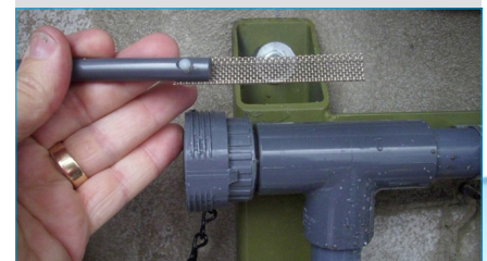
Checking System Corrosion Rates with the Use of a Coupon Rack
