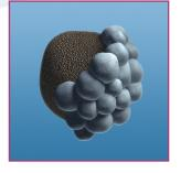
Without the surface charge, CaCO<sub>3</sub> will plate out around the particles rather than scale on the equipment surfaces. Two reasons it does this:
