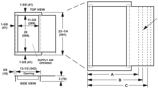
Break off extended width at pre-perforated line to fit specific air handler application.
